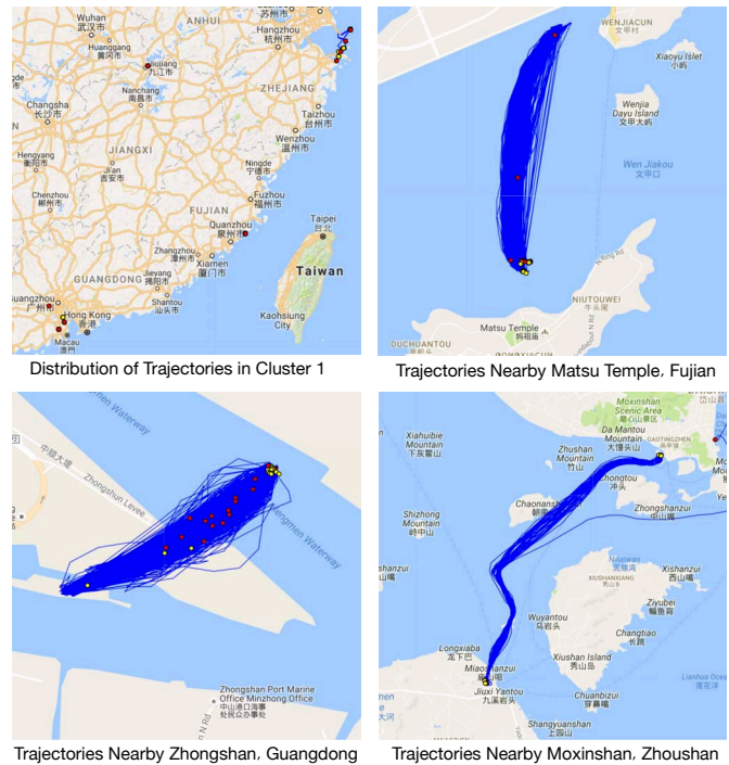
Fig. 10. Trajectories in Cluster 1. The blue lines stand for the trajectories; the yellow points stand for the start point and the red points stand for the end point. Most of trajectories in this cluster are short round trips between tourist cities and generated by passenger ships .
